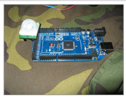
• GND to ground, V+ to pin 53, OUT to pin 51.
